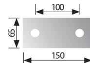
Fixing Holes to be 18mm in diameter U.N.O.
